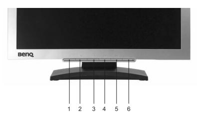
There are 6 keys for user's control including "*iKey*", "Exit", "Enter", "<" and ">" key and a power swith. The following descriptions are the introduction of these keys & switch.
